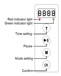
Press the "M" button on the control panel to select the wavelengths you want. You can choose red, display"R" or Near infrared, dispay"I". Or Both that display"RI"
